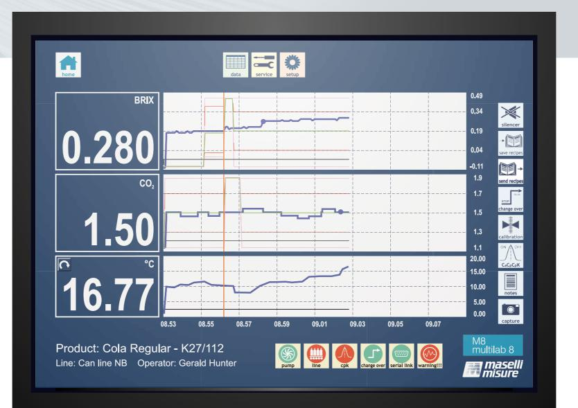
High performance diagnostic software notifies the operator of any problems; the operator need only to press a button to memorize all the line operating parameters active at that precise moment so that they can be passed on to our technical assistance service to help rectify the problem as quickly as possible.
